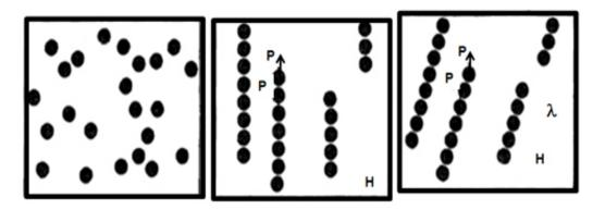
**Ans:** M. R. Particles are iron particles. In most of devices (i.e. damper, brake, engine mounts), these particle are subject to relative sliding motion, therefore cause three body abrasion. To reduce the three body abrasion, particles are made in spherical shape. Functioning of M.R. particle is illustrated in a set of three figures shown above. First figure indicates the dispersion of micron sized iron particles in liquid
